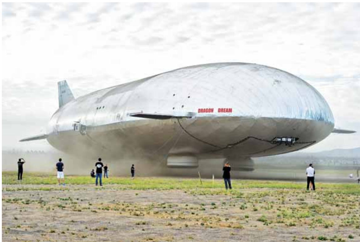
The Dragon Dream, a prototype of a lighter-than-air cargo airship built by Worldwide Aeros Corp., lifts off in its first flight at the Marine Corps Air Station in Tustin, California, in August 2013. The blimp is 81 meters in length and 30 meters wide, and incorporates a revolutionary new buoyancy control system. (Worldwide Aeros Corp.)
